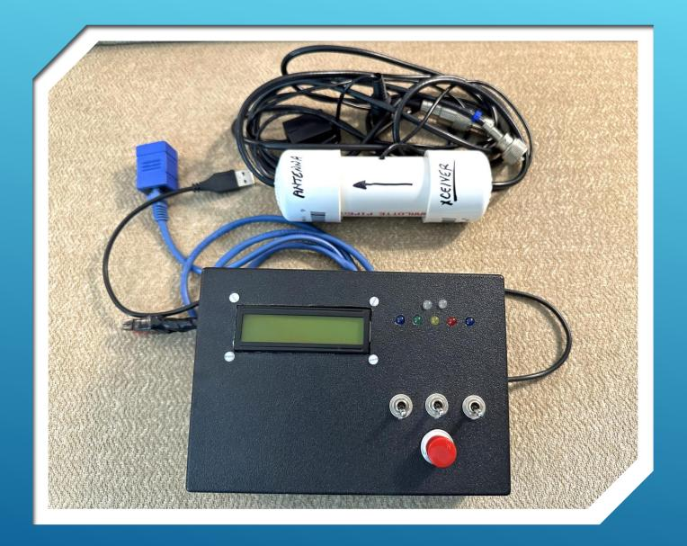
> Magnetic-Loop Antenna Tuner
